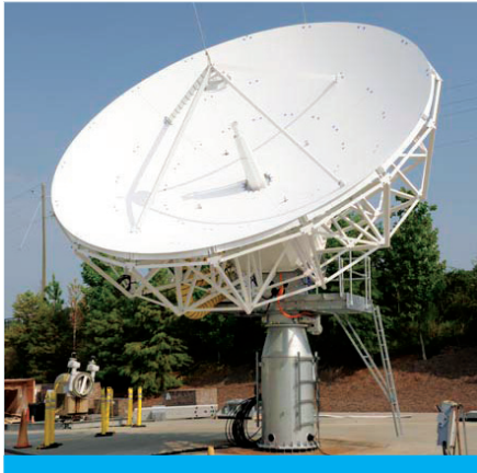
Gateway Antenna ready for Factory Acceptance Testing
